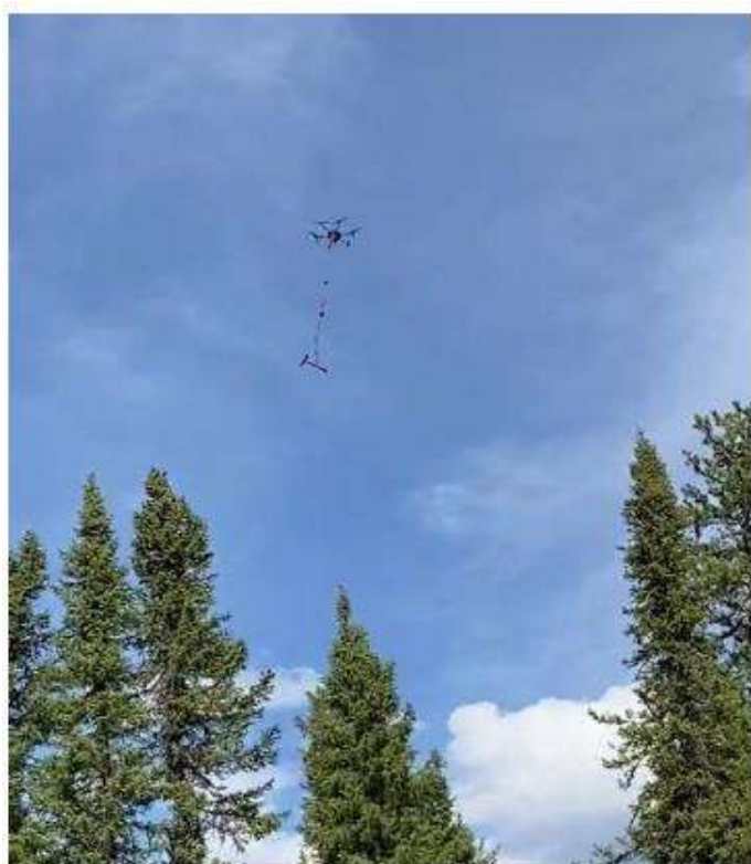
Figure 10. A magnetometer towed by a UAV or drone measuring the magnetic signature of the rocks on the ground over the Zoro Lithium Property.
