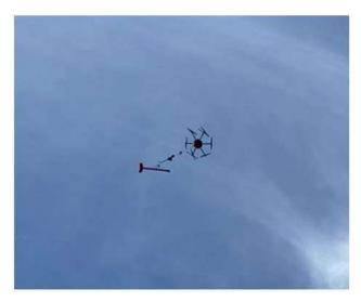
Picture 2. Drone Carrying a Magnetometer.
