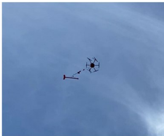
Picture 2. Drone Carrying a Magnetometer
